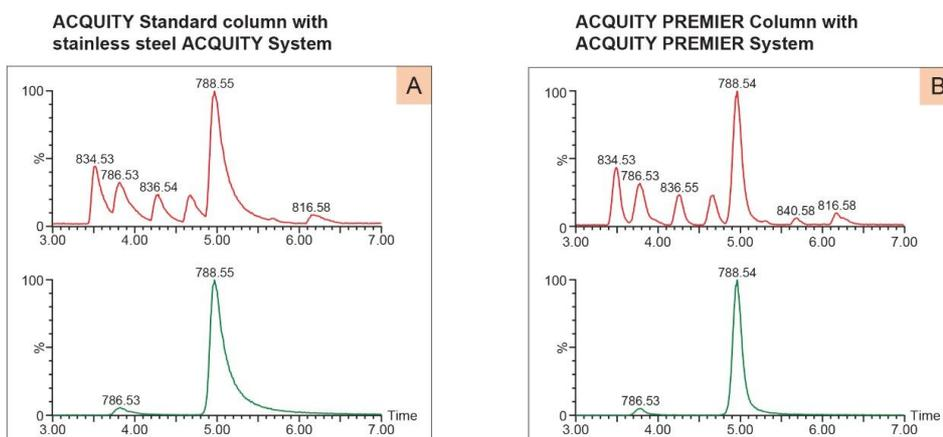
Figure 5. Avanti polar lipids brain porcine PS extract (10 µg/mL) measured using (A) ACQUITY standard CSH C<sub>18</sub> Column with stainless steel surface ACQUITY System (B) PREMIER CSH C<sub>18</sub> Column with ACQUITY PREMIER System. The bottom panel shows extracted ion chromatogram for PS (18:0\_18:1) at m/z 788.54 with peak width 1.1 min for standard CSH C<sub>18</sub> Column with stainless steel and 0.3 min for PREMIER CSH C<sub>18</sub> Column with ACQUITY PREMIER System.
