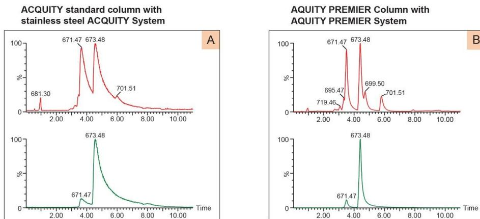
Figure 4. Avanti polar lipids egg chicken PA extract (10 µg/mL) measured using (A) ACQUITY standard CSH C<sub>18</sub> Column with stainless steel surface ACQUITY System (B) PREMIER CSH C<sub>18</sub> Column with ACQUITY PREMIER System. The bottom panel shows extracted ion chromatogram for PA (16:0\_18:1) at m/z 673.48 with peak width 4.1 min for standard CSH C<sub>18</sub> Column with stainless steel system and 1.2 min for PREMIER CSH C<sub>18</sub> Column with ACQUITY PREMIER System.
