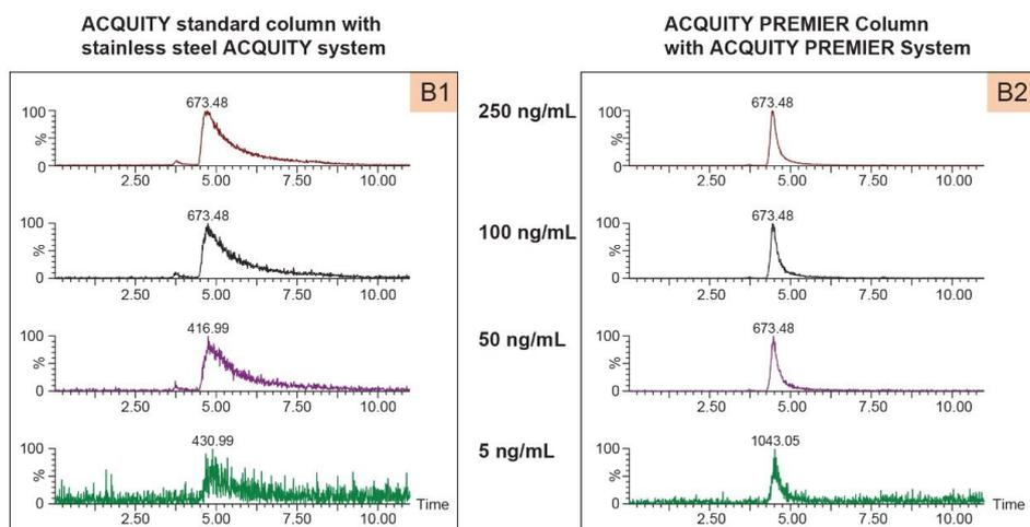
Figure 2B. Negative mode base peak extracted ion chromatogram of PA (16:0/18:1)  $m/z$  673.4808 at a concentration of 5, 50, 100, and 250 ng/mL. (B1) using ACQUITY standard CSH  $C_{18}$  Column with stainless steel surface ACQUITY System and (B2) using PREMIER CSH  $C_{18}$  Column with ACQUITY PREMIER System.
