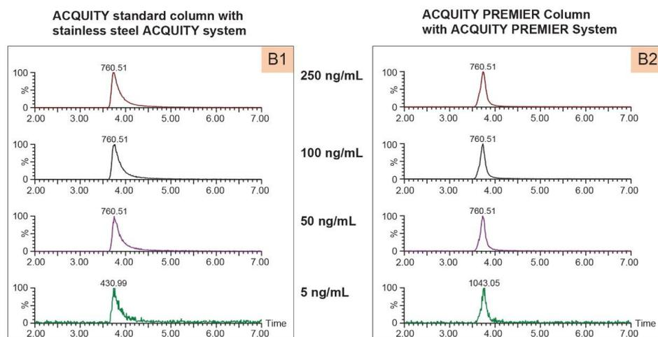
Figure 3B. Negative mode base peak extracted ion chromatogram of PS (16:0/18:1)  $m/z$  760.5129 at a concentration of 5, 50, 100, and 250 ng/mL. (B1) using ACQUITY standard CSH  $C_{18}$  Column with stainless steel surface ACQUITY System and (B2) using PREMIER CSH  $C_{18}$  Column with ACQUITY PREMIER System.
