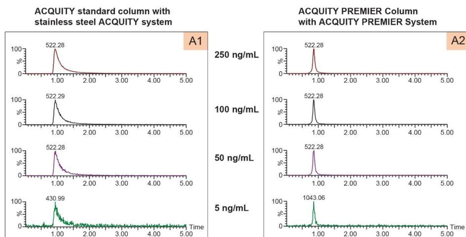
Figure 3A. Negative mode base peak extracted ion chromatogram of LPS (18:1/0:0)  $m/z$  522.2832 at a concentration of 5, 50, 100, and 250 ng/mL. (A1) using ACQUITY standard CSH  $C_{18}$  Column with stainless steel surface ACQUITY System and (A2) using PREMIER CSH  $C_{18}$  Column with ACQUITY PREMIER System.
