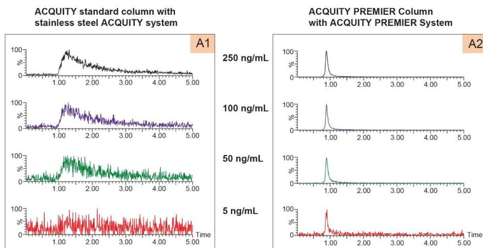
Figure 2A. Negative mode base peak extracted ion chromatogram of LPA (16:0/0:0)  $m/z$  409.2355 at a concentration of 5, 50, 100, and 250 ng/mL. (A1) using ACQUITY standard CSH  $C_{18}$  Column with stainless steel surface ACQUITY System and (A2) using ACQUITY PREMIER CSH  $C_{18}$  Column with ACQUITY PREMIER System.
